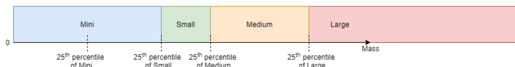
Figure 4: A diagram demonstrating how missing segments are imputed by matching a vehicle's average mass to the 25th percentile of known segments' mass.
