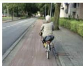
Figure 30. Separated Cycle Paths – the Netherlands uses red colour and texture on its cycle paths throughout the country so inhabitants are clear on the distinction between cycle paths and pedestrian paths. (Photo: Tim Jones)
